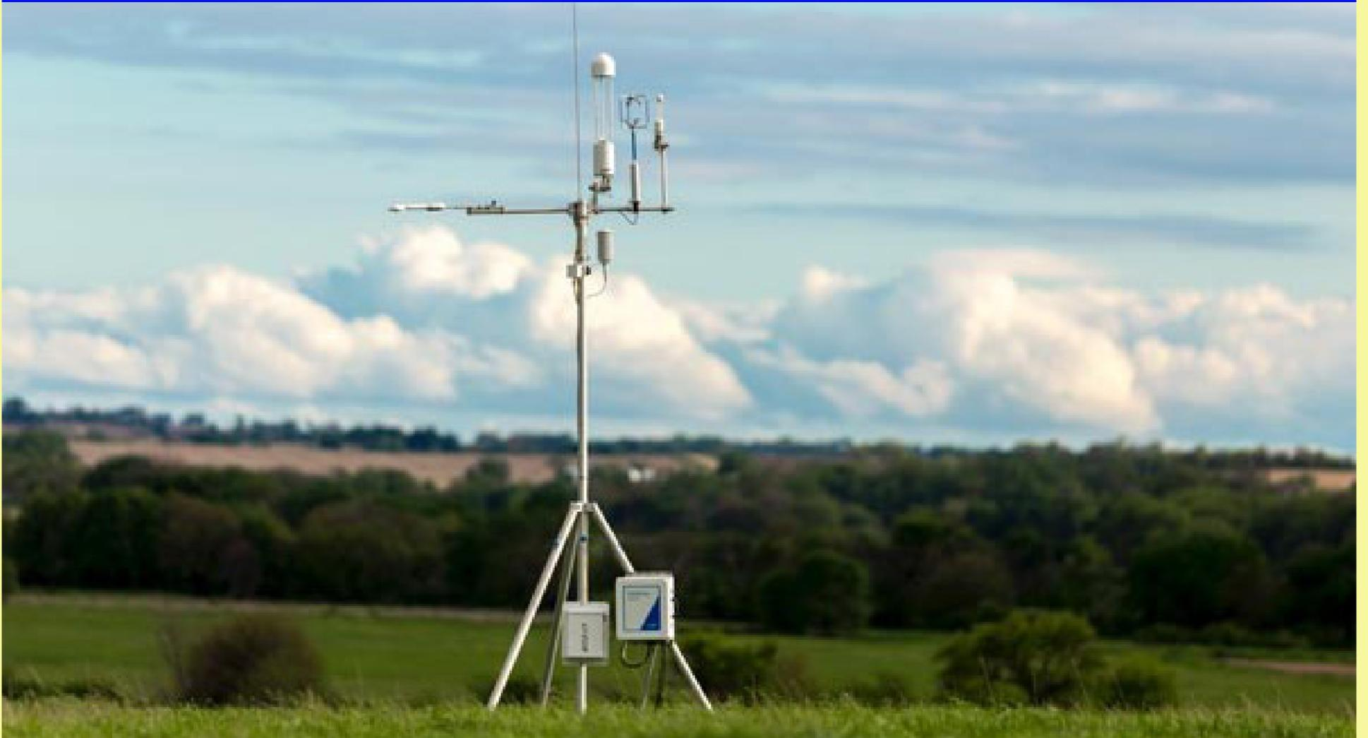
*Eddy covariance flux tower for atmospheric measurements*
